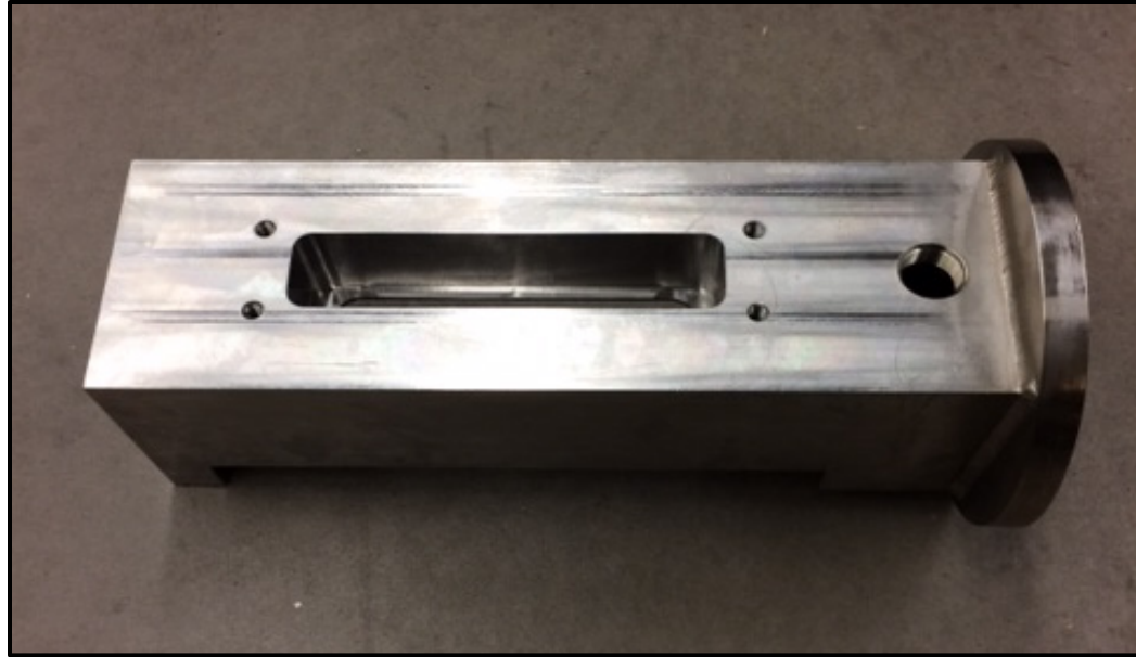
Figure A-15 (a) Top View and (b) Bottom View of the test-section housing with the exit flange welded to it.
