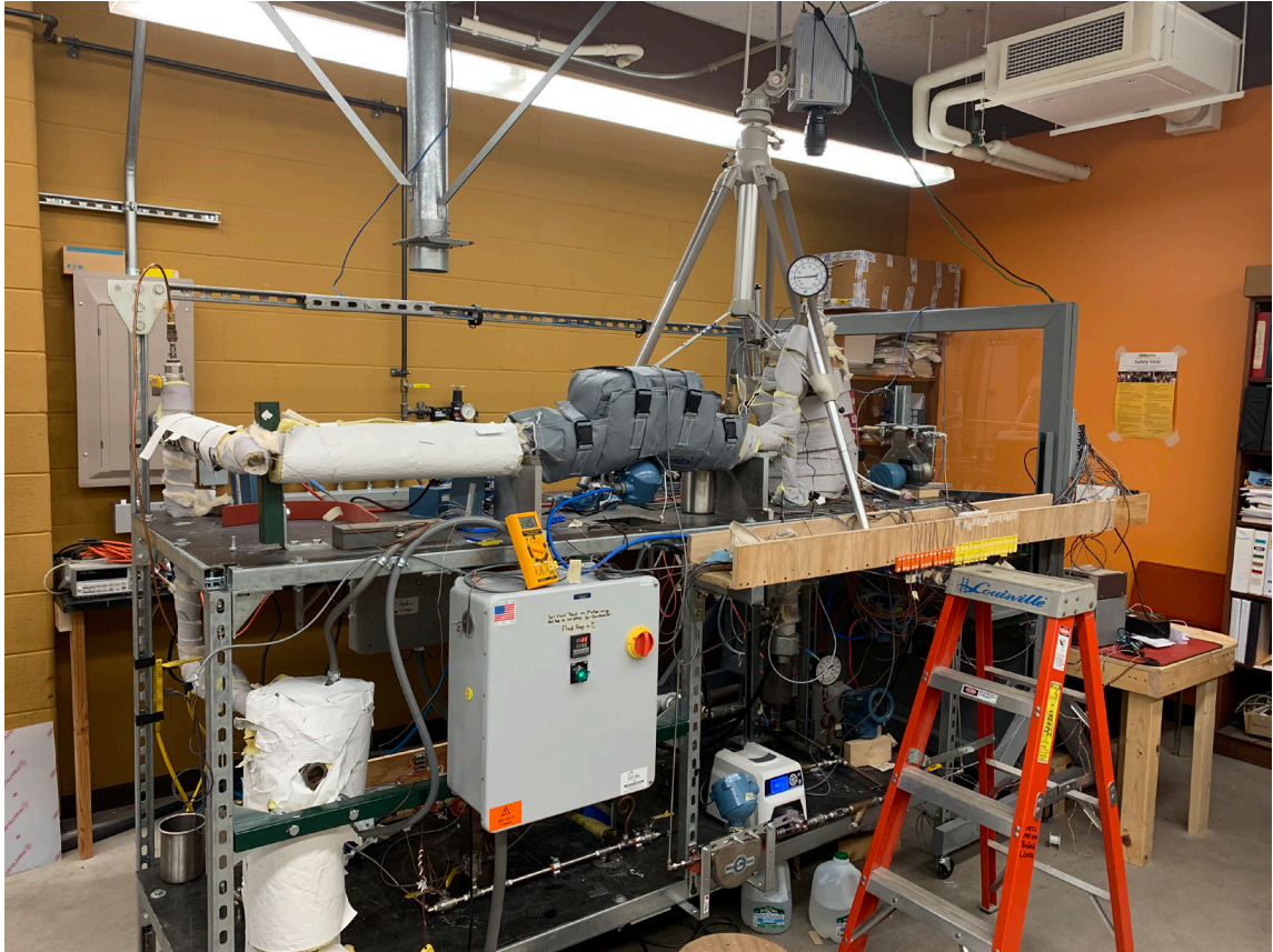
Figure A-2 The flow loop physical set-up during a test run on December 27 th 2018. The high-speed camera is set up at the top of the tripod facing and adjusted in the flow channel during the run.
