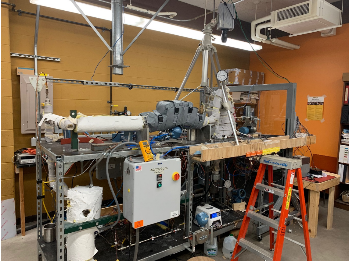
Figure 3-4 The flow loop test stand and equipment
